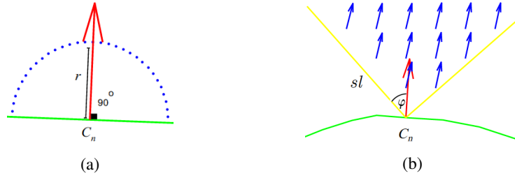
Figure 1: (a) Region S and (b) T for snake element C_n . The snake, the direction of F_{Balloon} , and the GVF field vectors are represented in green, red and blue, respectively.
