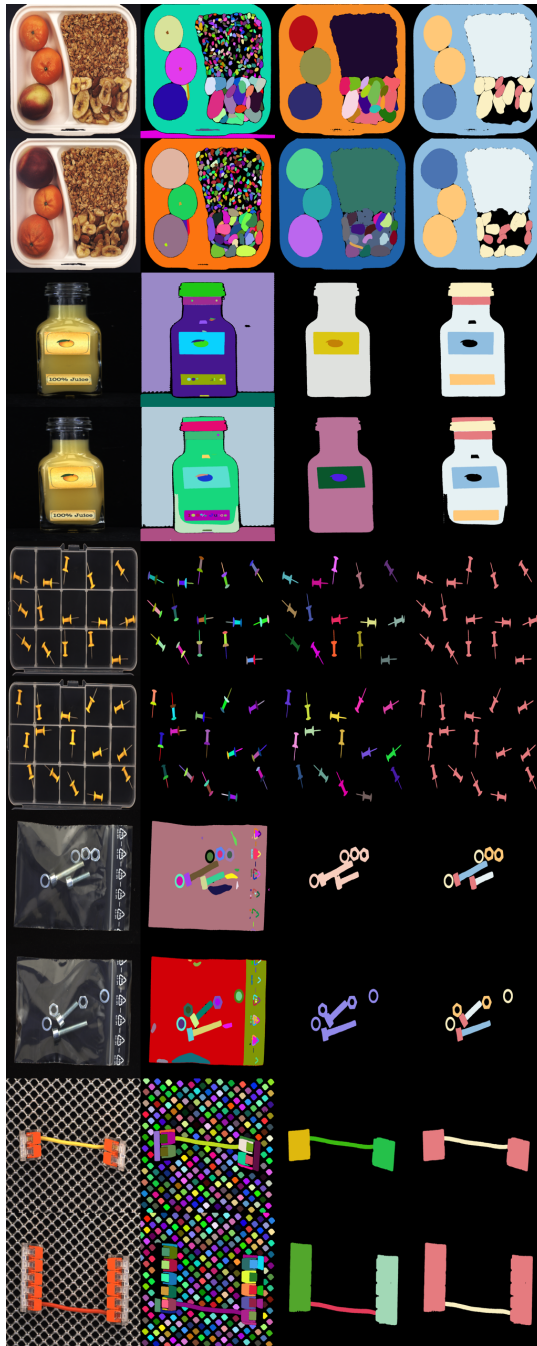
Figure 6: Example images of pseudo label generation of the five categories of the MVTecc LOCO, from left to right, represent normal image, X^{seg} , X^{sem} , and pseudo label image. In each category, random colors are assigned to different masks in X^{seg} and X^{sem} while the same color represents the same class in the pseudo-label image.
