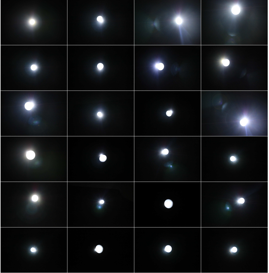
Figure 3: Samples of 80 different flare patterns captured in a dark room setting to enhance our FMG network’s performance by reducing the gap between the training and test datasets
