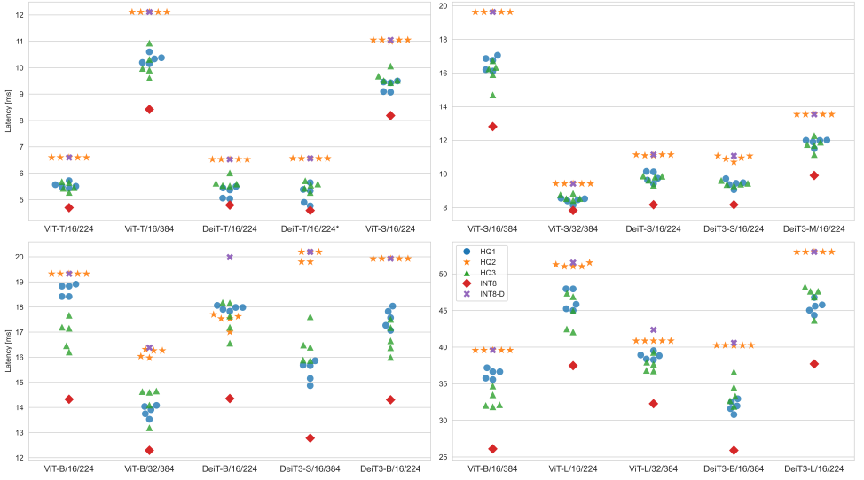
Figure 1: CPU-only workstation: Average Intel Xeon 5218 Gold CPU inference latency of models. Each point represents a single quantization configuration. We report the average latency of linear layers over 1000 samples.
