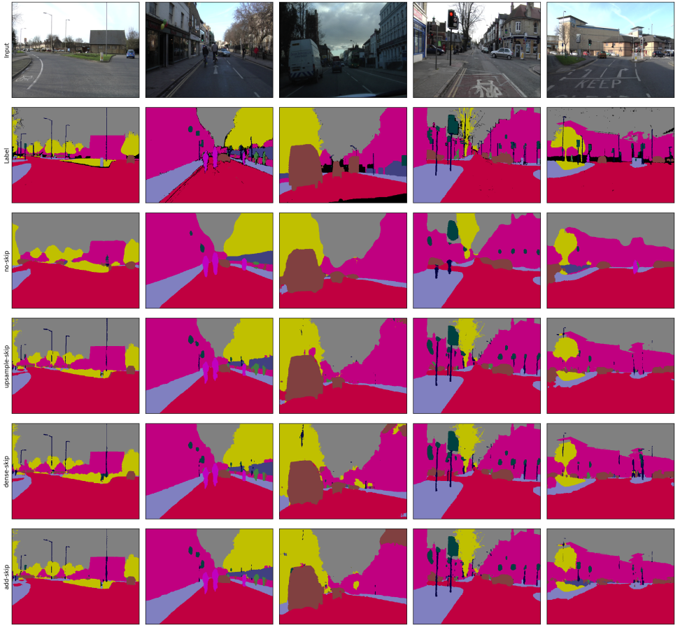
Figure 8: Qualitative results of modifications to skip connections. We highlight that no-skip produces very coarse results with smooth boundaries, as it’s unable to recover the spatial resolution without the skip connections. On the opposite spectrum, dense-skip is able to better predict small and thin classes such as posts and signs.
