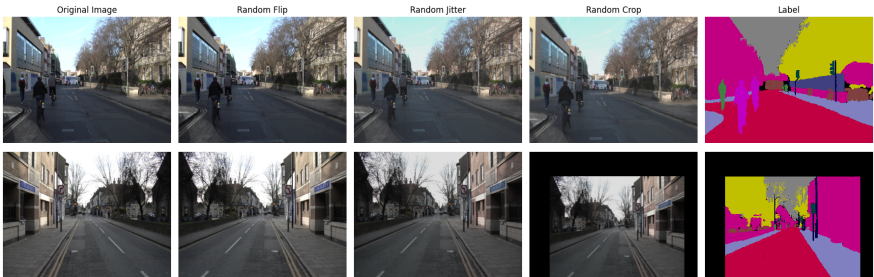
Figure 5: Example of two images going through the augmentation process step by step, the images are randomly flipped, jittered, and cropped. Note that the label and the image go through the same augmentation but with random parameters each time. Image augmentation is computed in parallel to the main training loop
