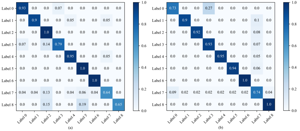
Figure 4: (a) Confusion matrix for MobileNetV3, (b) Confusion matrix for ML-2SN. Label 0 to Label 8 in the confusion matrix are, in order, lying down, right body lean, left body lean, head forward, right head tilt, left head tilt, right-hand support, sitting normally, left-hand support.
