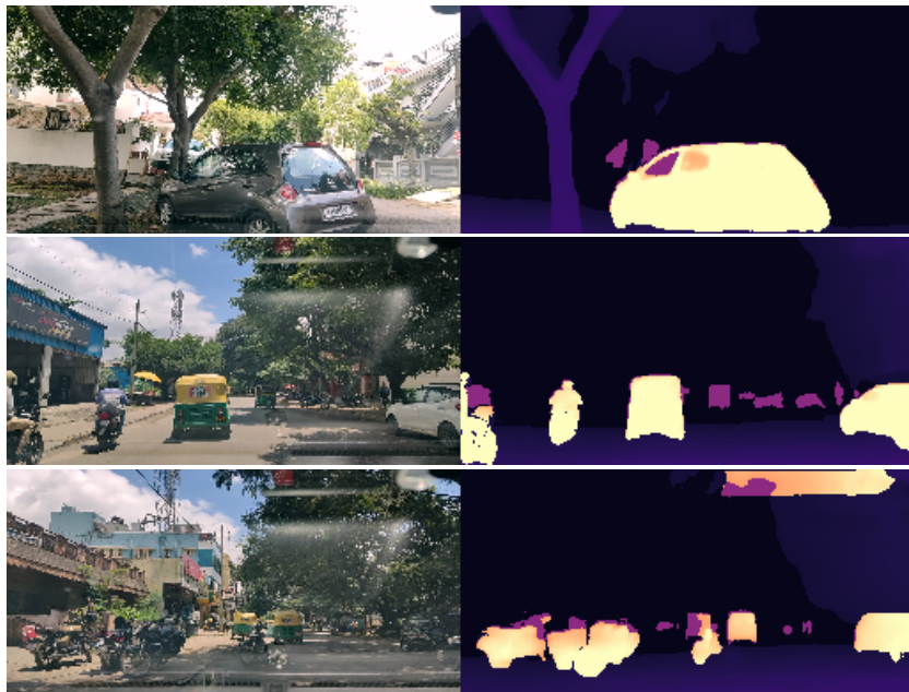
Figure 2: Importance Maps. The first column shows the input video frames and the second column presents the corresponding importance maps, with the entire scene’s importance scaled from zero to one as a function of distance and semantics.
