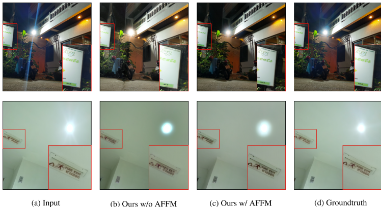
Figure 4: Visual comparison on the effect of AFFM. Without AFFM, SGIM can effectively remove lens flare, but there are significant distortions on flare-free areas. When AFFM is employed, the fidelity of flare-free areas has been maintained between the input image and the restored image.
