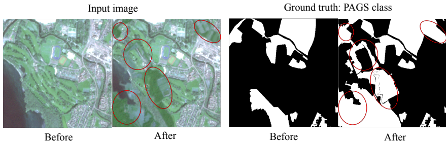
Figure 2: Copy-Paste example. Left: input image before and after Copy-Paste, right: ground truth mask for PAGES class (white for true and black for false) before and after Copy-Paste. Red lassos highlight the pasted PAGES pixels.
