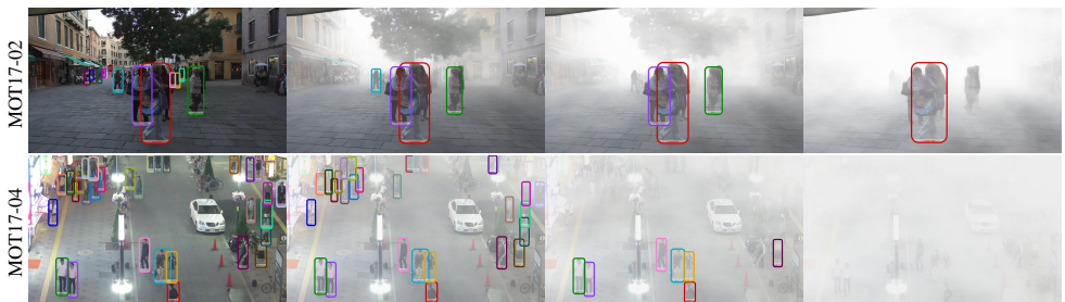
Figure 1: Visualization of MOT performance degradation with increasing fog intensity (from left to right), demonstrated on fog-augmented video sequences with different scenarios. Top row: a daytime front-view static camera scene. Bottom row: a heavily illuminated night crowd surveillance scene. (Best viewed on screen.)
