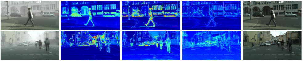
Figure 3: Col 1: input images. Cols 2 – 4: learned foreground attention masks. Local-global self-supervision accentuates semantic object content regions and improves translation in areas critical for object detection (e.g. people, cars). Col 5: translated output images.
