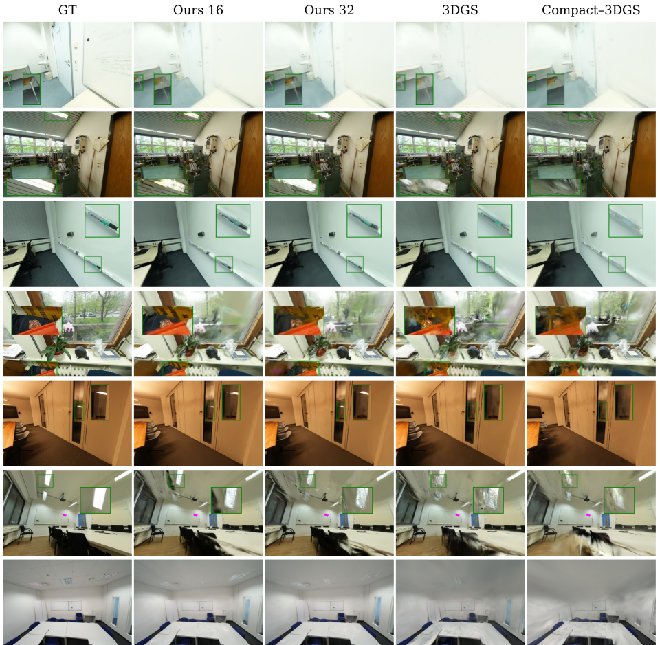
Figure 6: Novel view synthesis of FeatSplat–16 and FeatSplat–32, against 3DGS [9] and Compact-3DGS [17] on a subset of scenes from ScanNet++ [38].
