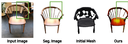
Figure S8: Limitation of model dependencies. The green square indicates object occlusion in the input image, which disrupts segmentation, leading to the disappearance of the reconstruction mesh.
