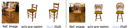
Figure 6: Necessity of pre-optimization for radius. The “w/o pre-optim.” cases exhibit geometry cut-off for exceeding the camera space boundary and degradation of details.
