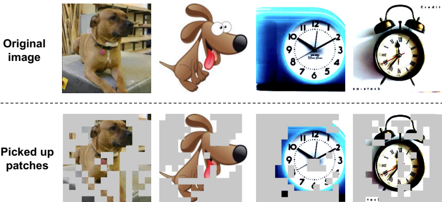
Figure 3: Visualization of picked up patches. The original images and the regions that the model picks up to minimize the entropy are shown. The patches that are not selected by the model are colored in gray. We can see that the model correctly selects the regions that possess strong class information.
