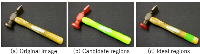
Figure 1: The difference between candidate regions and ideal regions. Green and red show the regions that can be grasped and can pound, respectively.
