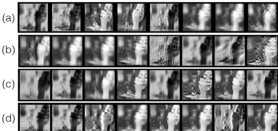
Figure 2: Comparison of layer activation of the first convolution layer for (a) 3D convolution, 1st stream (b), 2nd stream (c), and 3rd stream (d) of P_3SC_1 layers.
