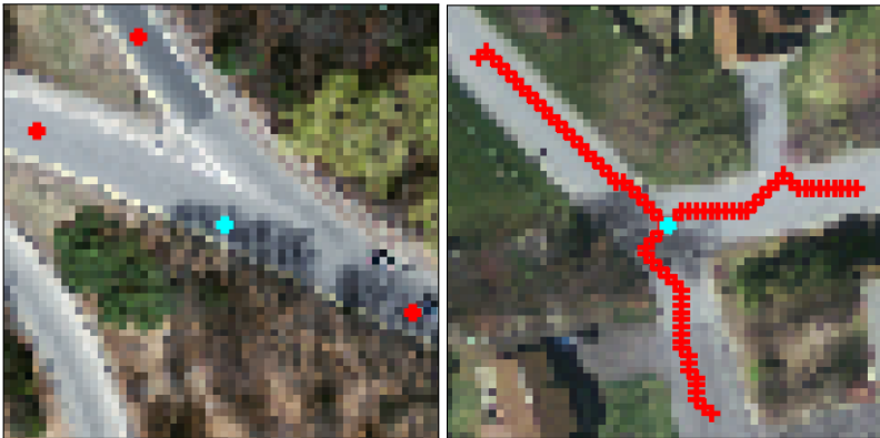
Figure 2: Left : Example of training patch for connectivity. The red points represent the locations from the patch border connected with the road indicated by the blue point in the center of the patch. Right : Shortest path on semantic segmentation to connect the locations detected at the patch border with the patch center.
