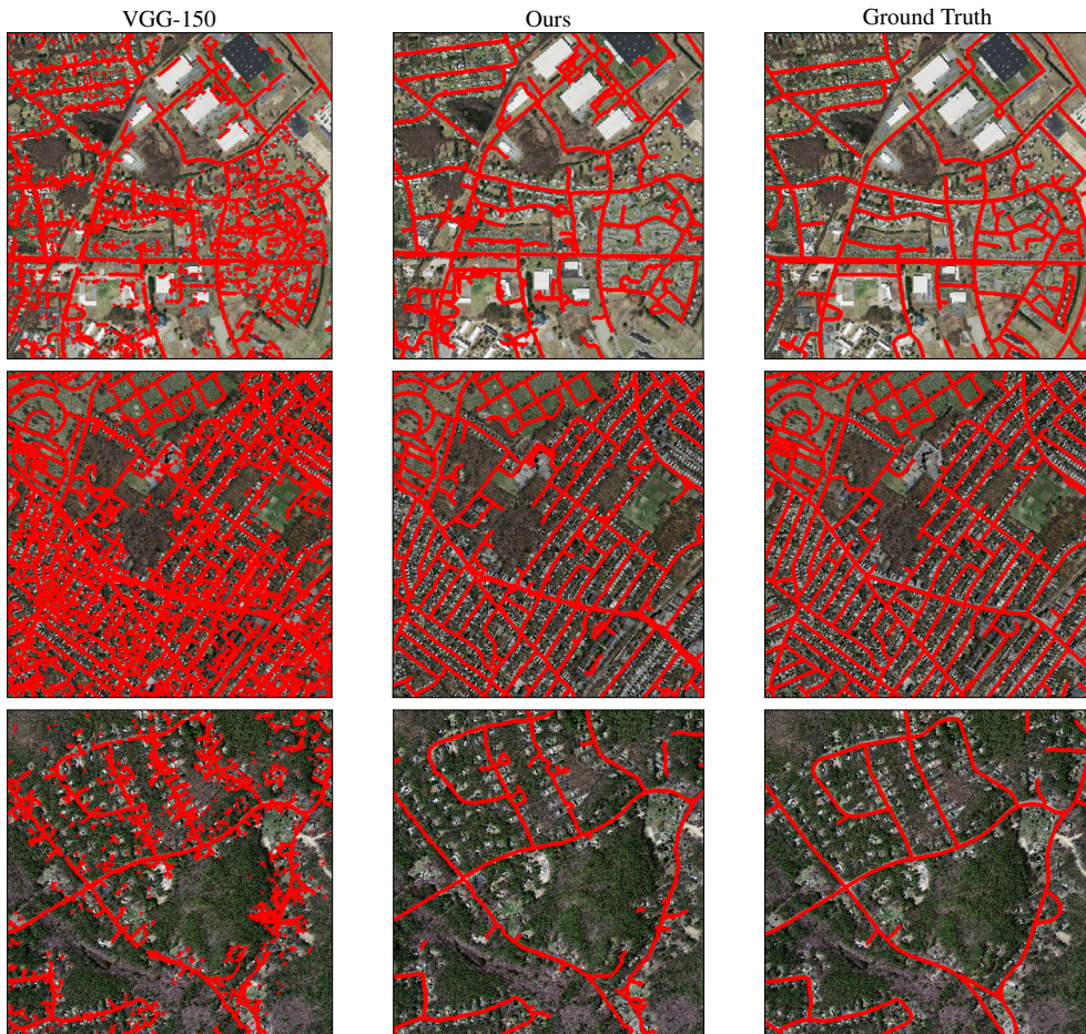
Figure 6: Results for road network topology extraction on the Massachusetts Roads dataset. From left to right: VGG-150, our iterative delineation approach and ground truth.
