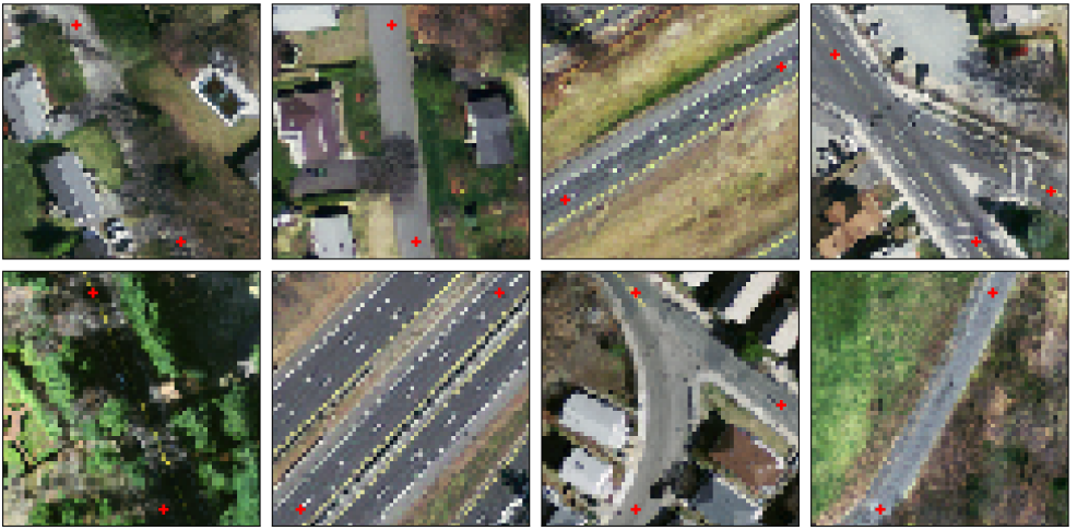
Figure 3: Visual results for the patch-level model for connectivity applied to patches from the Massachusetts Roads dataset. The red crosses represent the detections.
