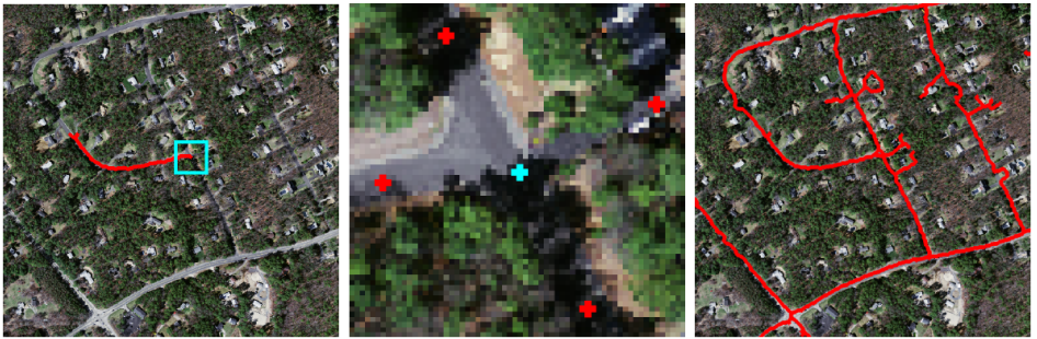
Figure 1: Patch-based iterative approach for network topology extraction. Left : Current state at some point of the iterative approach where the patch-level model for connectivity is applied over the blue square. Center : Detections at the local patch for the points at the border (in red) connected to the central point (in blue). Right : Final result once the iterative approach ends.
