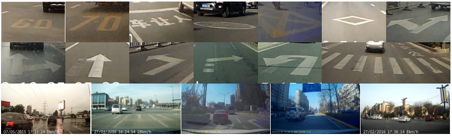
Figure 1: Examples of road markings in our dataset. The first two lines show 13 categories of road markings. From left to right and top to bottom, they are 60, 70, car_people, center_ring, cross_hatch, diamond, forward_left, forward_right, forward, left, and right. The last line shows some images describing different traffic scenes.
