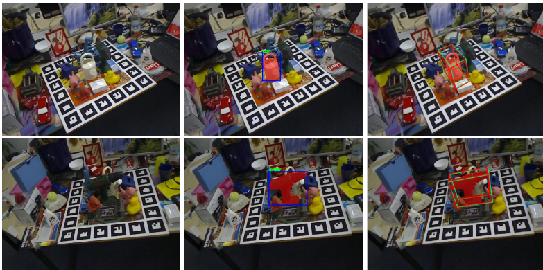
Figure 2: Some qualitative results of LieNet on the LINEMOD dataset [9]. Left: original images; Middle: predicted 2D boxes, classes, and segmentations; Right: green and red boxes are the groundtruth poses and predicted poses, respectively.
