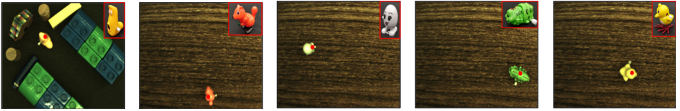
Figure 7: Results for naïve object tracking. We use wind-up toys as moving objects against a static background. Close-up shots of the tracked objects are shown in the top right corner of each image. The predicted position (red dot) is correctly identified within a maximum error rate of 6.78% with an average error rate of 2.82%. The complete video results for all toys are provided in the supplementary material.
