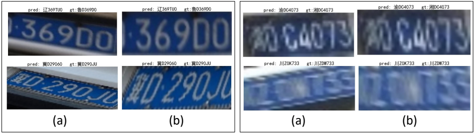
Figure 3: Visualized failure cases (a) Original patches (b) Rectified results. The "pred" are all predicted by our recognizer
