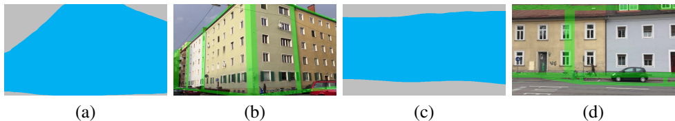
Figure 4: Façade only segmentations (a, c) and registration with our method overlaid over the input frame (b, d). The pair (a, b) shows a configuration where segmenting the façades alone is sufficient for successful tracking, while for the pair (c, d), additional constraints from the edges would be required.
