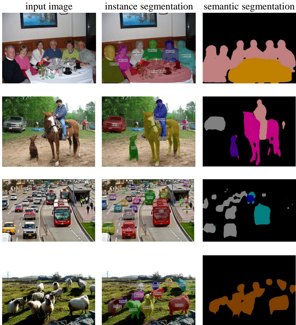
Figure 5: Results of BiSeg. Our method produces high segmentation quality at borderlines without using CRF. For instance segmentation, we show all detected instances whose classification scores are larger than 0.5. We confirm good results of instance segmentation even for heavily occluded scenes (the last two rows).
