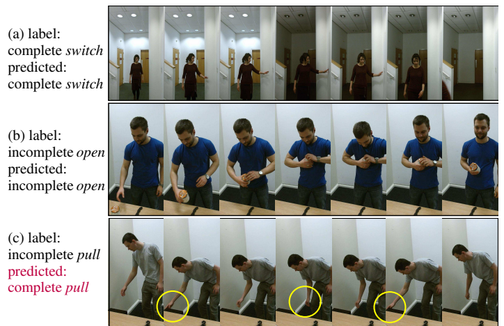
Figure 2: Sample frames of correctly (a), (b) and incorrectly (c) classified test sequences. In (c), using JV solely, the hand seems to perform a pull in full even when the drawer remains unmoved.
