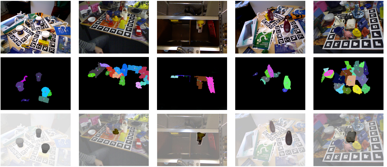
Figure 2: Examples of the approach on different images. First row: RGB images; second row: segmented objects; third row: detected object superimposed.
