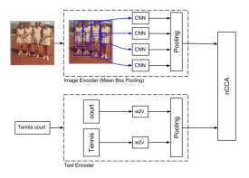
Figure 1: Overview of our full model, i.e. our proposed image representation using Mean Box Pooling, text encoding using average of Word2Vec representations, and normalized CCA for learning the joint space.
