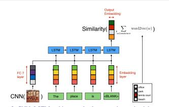
Figure 2: CNN+LSTM architecture that learns to choose the right answer directly in the embedding space. The output embedding is jointly trained with the whole architecture via backpropagation.
