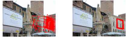
Figure 2: In this scene the pose cannot be accurately estimated with a standard RANSAC-PnP approach (left). Patch synthesis improves the registration of the query view to the scene, as proved by the superposed scene edges (right).
