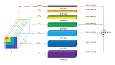
Figure 2: The illustration of scale pooling technique for BoSP (We can extract different number of features from 7 scales. For example, there are 49 red strips for the smallest scale, and only 1 purple strip for the largest scale. Then we max pooling the features inside each scale and add up to form the final feature).
