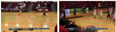
Figure 2: Sports camera calibration examples, best viewed in color. The court lines are overlaid on the images to indicate the accuracy of calibration.
