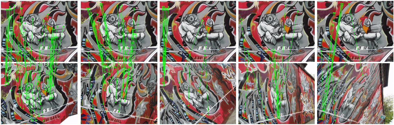
Figure 9: Qualitative evaluation of feature transferability: Keypoint detection and matching results from network trained on aerial imagery and tested on “Wall” image from the Oxford dataset [19]. For the first two images the network successfully retrieves the correct homography. The result on the third is partly correct. The last two image demonstrate failure cases.
