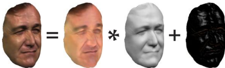
Figure 1: The reflected intensity is the product of albedo and diffuse shading plus specularities.
