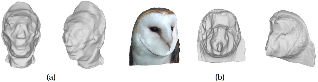
Figure 4: Examples of Poisson reconstructions: (a) shaded geometry from novel viewpoints from the face sequence (frame 1); (b) textured and shaded geometry from novel viewpoints from the barn owl sequence (frame 1).
