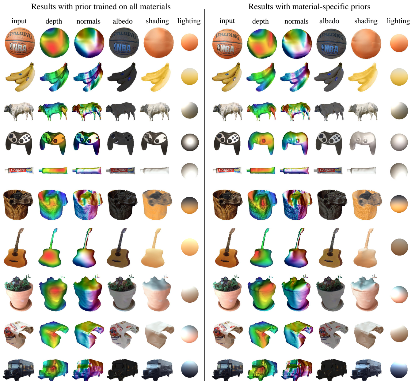
Figure 6: Visual comparison of results generated with a prior trained on all materials (left column) and with priors trained on the detected material category (right column). Each result consists of 6 images from left to right: the input image, estimated depth, normals, albedo, shading and lighting. Overall, the material-specific priors enable a better separation of the intrinsic factors and finer details are recovered. Best viewed digitally.
