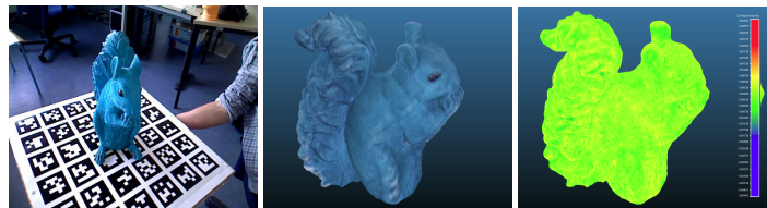
Figure 3: Example frame from one sequence, meshed result and reconstruction difference between the dense and the Octree version.
