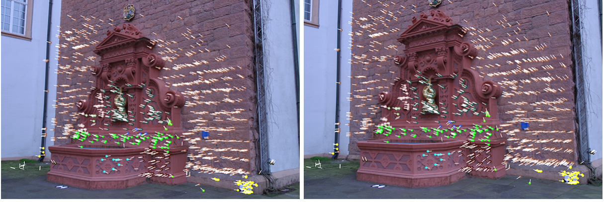
Figure 5: Correspondence clustering into tangent planes for frames 1, 2 of the fountain-P11 set. Planes denoted by colour, estimated surface normals visualized by white line segments.
