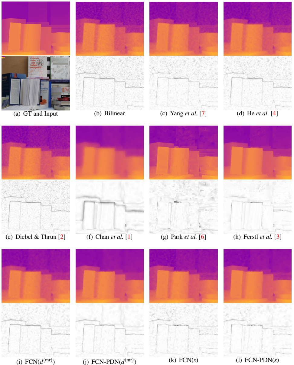
Figure 11: Qualitative results for the image Books from the noisy Middlebury dataset [6] and a scale factor of \times 16 . The first image in (a) shows the ground-truth HR depth and the second image depicts the input sample. In (b)-(l) we present the HR estimates of various methods and the corresponding error maps.
