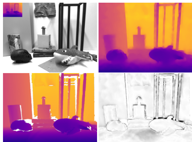
Figure 2: Qualitative results for the Shark dataset from the ToFMark benchmark [2]. The first row shows the input and the output of our method, respectively. In the second row we present the ground-truth depth and the error of our method.
