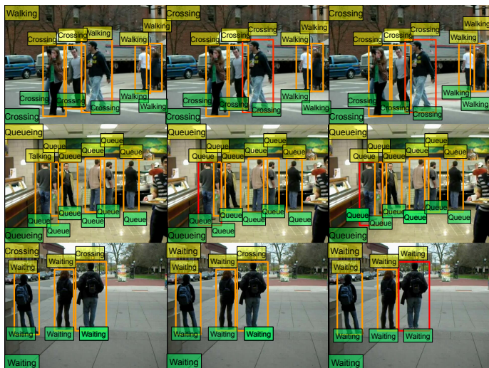
Figure 4: Results visualization for our model. Green tags are ground truth, yellow tags are predicted labels. From left to right is without message passing, first step message passing and second step message passing
