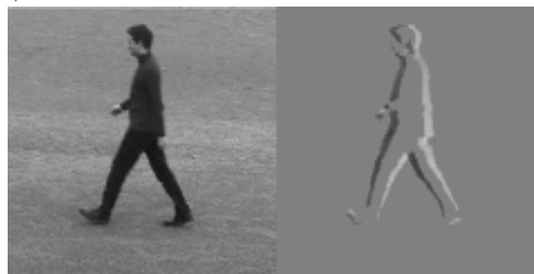
Figure 4: Left: a frame from a video from the Recognizing Human Actions video dataset. Right: the difference between that frame and the previous frame, with thresholding applied to increase sparsity. Stacking the frame differences produces a sparse 2+1 dimensional space-time object.
