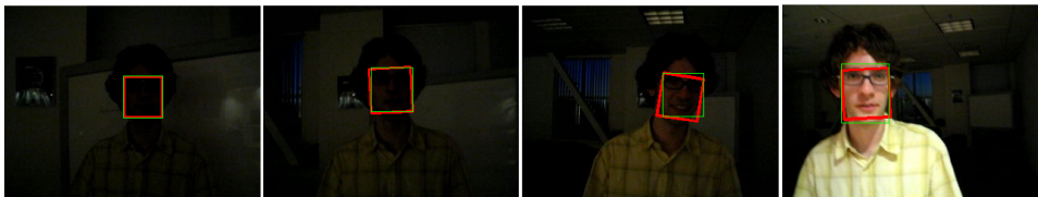
Figure 5: Robustness towards illumination changes is achieved by normalising the patches extracted from the image. Even in sequences like ‘David’, where extreme illumination changes are present, our method performs correctly.
