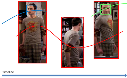
Figure 3: Face tracks (blue and green) and a person track (red) are merged into one track node.
