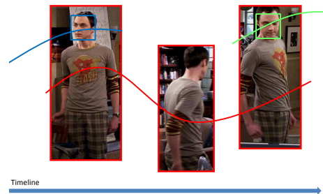
Figure 2: Face tracks (blue and green) and a person track (red) are merged into one track node.
