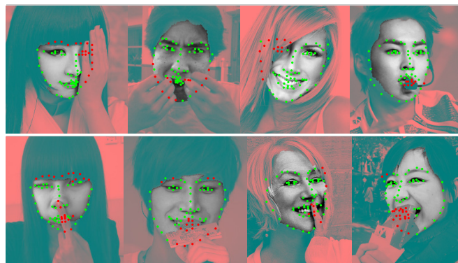
Figure 2: Examples of landmark localization, occlusion, and segmentation mask estimation for images from the COFW test data produced by our model.
