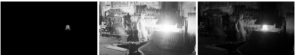
Figure 3: Comparison of complete histogram equalisation and proposed method. From left to right: linearly scaled HDR image, result of complete histogram equalisation of the HDR image, result of constrained histogram equalisation (proposed first stage) applied on the HDR image.
