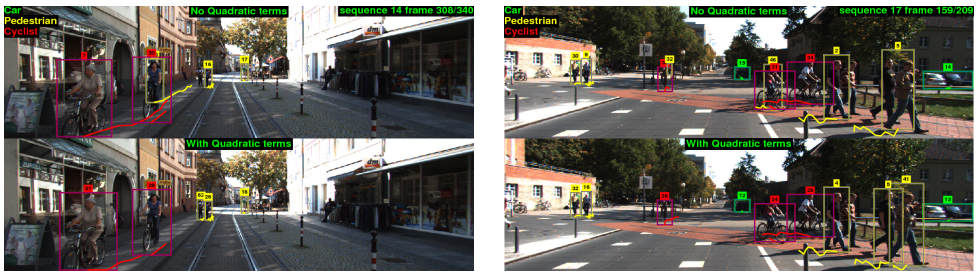
Figure 1: Our tracking framework incorporates quadratic interactions between objects in order to resolve appearance ambiguity and to boost weak detections. The parameters of the interactions are learned from training examples, allow the tracker to successfully learn mutual exclusion between cyclist and pedestrian, and boost to intra-class co-occurrence of nearby people.
