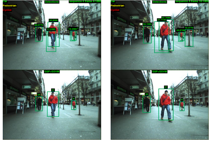
Figure 1: By learning a proper set of parameters, even a basic network-flow model without pairwise potentials can successfully prune away many false tracks by reasoning about detection confidence and transition smoothness.
