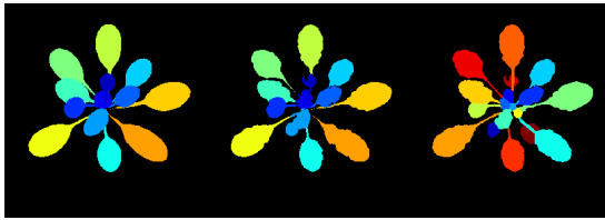
Fig. 2: Example segmentation output by our algorithm (best viewed in color). Left: Raw segmentation. Middle: Segmentation after applying foreground mask. Right: Ground truth segmentation. Most errors result from mistakes made by our initialization heuristic, which could be fixed by additional trans-dimensional moves. For example, few interior leaves are found, which could be corrected by adding random birth moves.
