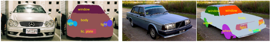
Figure 1: The goal of car parsing is to detect the locations of semantic parts and to perform object part segmentation. The inputs (left) are images of a car taken from different view-points. The outputs (right) are the locations of the car parts – the wheels, lights, windows, license plates and bodies – so that each pixel within the car is assigned to a part.
