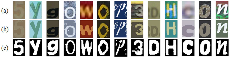
Figure 3: A few challenging examples of character images from ICDAR03-CH and Chars74k datasets where proposed method extracts and enhances the binary map of character region. (a) Input Images. (b) Quantized Images with 2-Colors MVQ. (c) Binary map of characters after noise reduction and enhancement.
